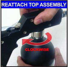
Screw top assembly onto canister in a clockwise direction. Make sure assembly has been fully seated.
