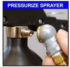
5. Charge sprayer with compressed air using a standard air chuck. Hold air chuck on valve stem until you hear the line pressure equalize with the sprayer.
