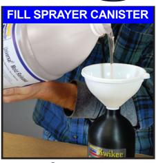
3. Fill Kwikee<sup>®</sup> sprayer no more than 2/3 full (24 oz/709 ml) maximum with a release or sealing agent that is clean and free of foreign particles.
