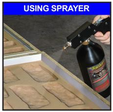
6. Working pressure is 80-120 psi. Maximum pressure should not exceed 200 psi. 80 psi is needed to spray the full 24 oz/709 ml.
